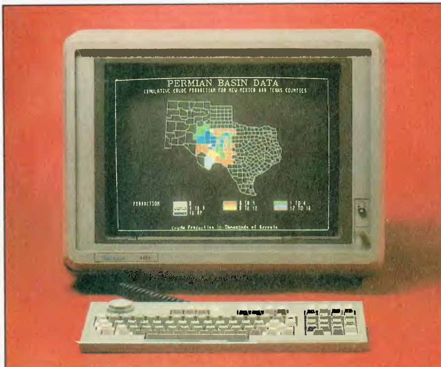
Tektronix's TEK 4109 computer display terminal has an addressable display matrix of 4096 by 4096, which allows the user to zoom in on a portion of the display.
